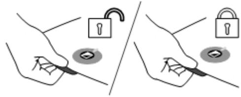
**Please note:** When the ClearView<sup>+</sup> power is off, the brake will automatically lock into position. When the ClearView<sup>+</sup> is switched on, the brake will unlock. Make sure to push the reading table backwards to its home position prior to turning off.
