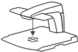
Pressing this button for three seconds will activate a red LED light, which shows as a red spotlight on the object in the centre of the reading table. It serves to indicate the centre of the on-screen image. To assist with writing, place a pen in the red spotlight on the reading table and see the pen displayed in the centre of your screen. Press this button once again to deactivate the LED light.
